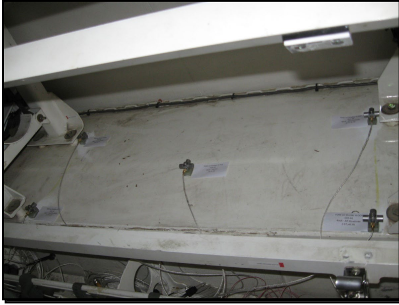
Figure 4. Transducer placement (input to missile rack).
