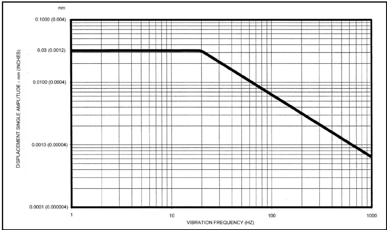
Figure 528.1-2. Vibration acceptance criteria for Type II vibration.
