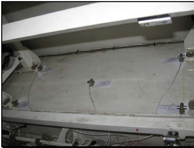
Figure 4. Transducer placement (input to missile rack).
